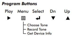
The Program buttons on the back of Algo 8180 allow local adjustment of alert tones and alert volume. The buttons are intentionally hidden from view after installation and can be disabled using the web interface. The button plays the current ring tone and allows volume adjustment using the V and A buttons.
